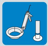
Prime penetrations using M-1<sup>®</sup> Universal Sealant/Adhesive, extending up 3 inches from the base and tool in. Apply three 1/4 inch diameter beads to the bottom of each curb section.
