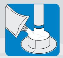
Fill curb with 1-Part<sup>®</sup> pourable sealer when installing around high movement details and on granulated surfaces.
