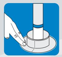
Press the curb in place. Seal around the joints and outside of the curb with a bead of M-1 and tool to ensure a monolithic seal.
